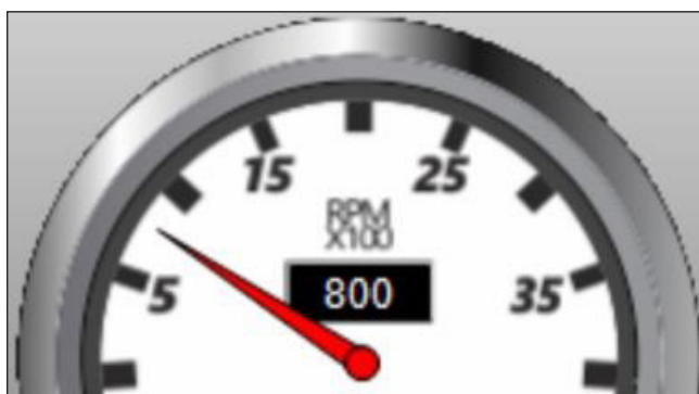
Figure 4.45 - Engine Speed Indicator
